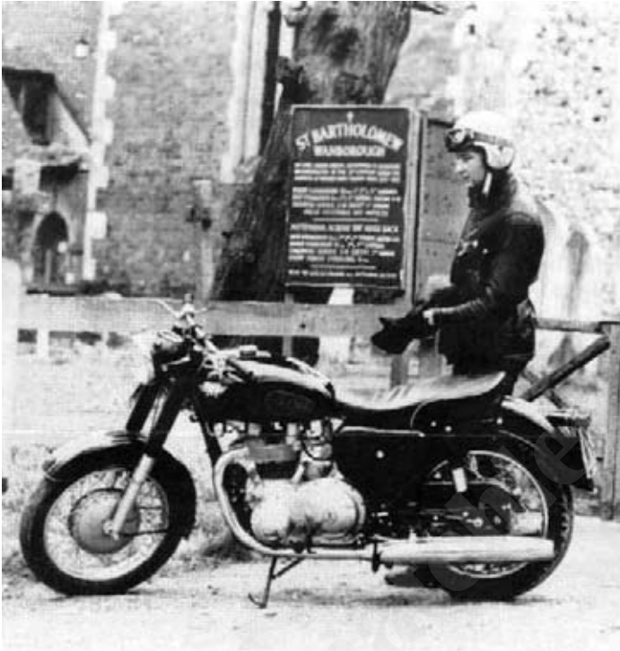
Matchless G12 Majestic with smaller tank badge for 1965 but otherwise little changed.
