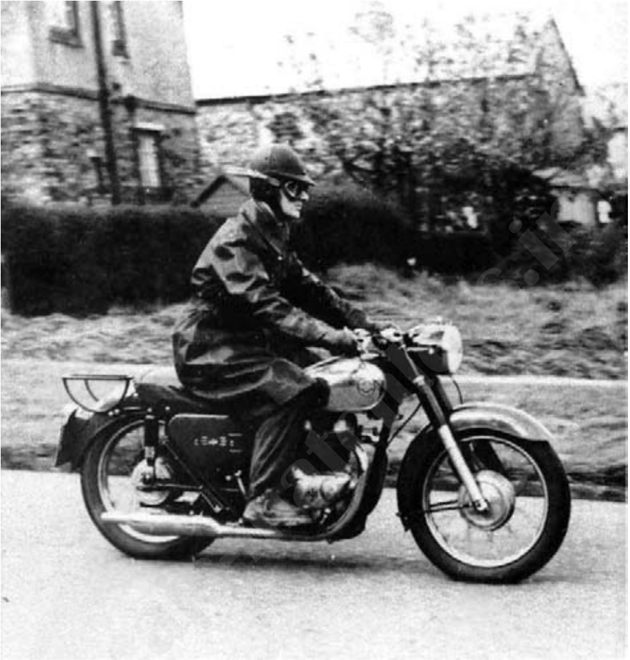
A 1959 AJS model 31 out on the road. This was the first year for the 646 cc twin and this standard one has alternator electrics.
