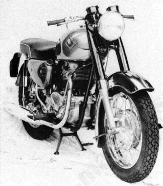
The 1966 AJS model 33 which used the Norton engine, forks and hubs while the gearbox had been common to AMC and Norton since 1957.
